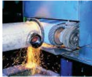
API's additional grinding process flattens tube ends and tubesheets which reduces risk of crevice corrosion, ensures even gasket compression and eliminates cracking of casting during manufacturing and servicing of units.
