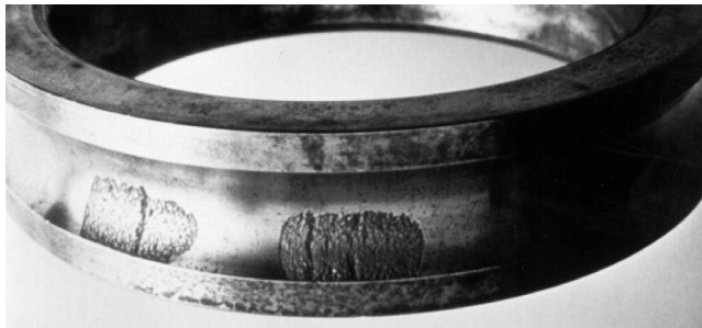
Figure 21. Two Load Zones on the Outer Race
