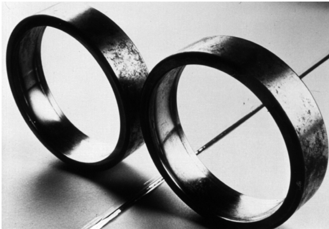
Figure 21. Two Load Zones on the Outer Race
