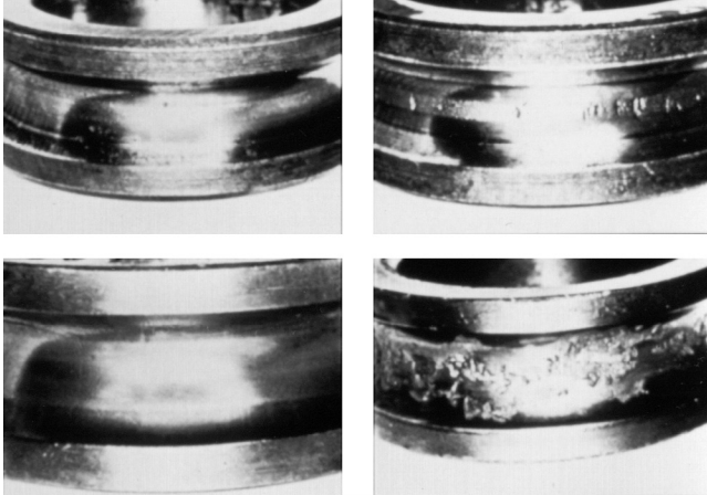
Figure 8. Progressive Failure of a Bearing Due to Inadequate Lubrication
