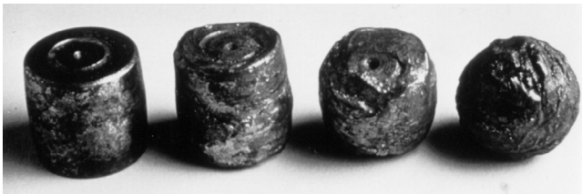
Figure 9. Damaged Spherical Bearing Rollers
