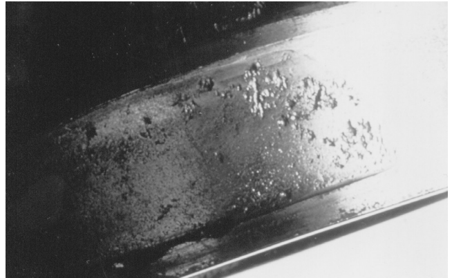
Figure 7. Spalls & Wear Patterns in the Race
