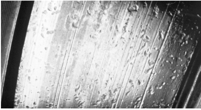
Figure 13. Severe Particle Denting
