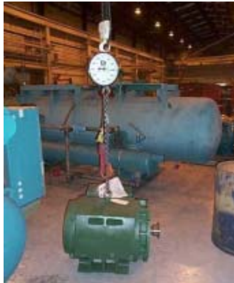
Figure 1. Weigh replacement motor.
