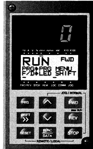
Figure 3-1-2 KEYPAD Panel Display with the Power ON
