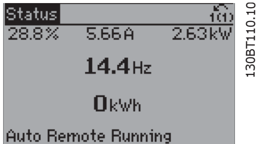
Illustration 2.7: Step 1: Turn on the frequency converter (green LED lights)
