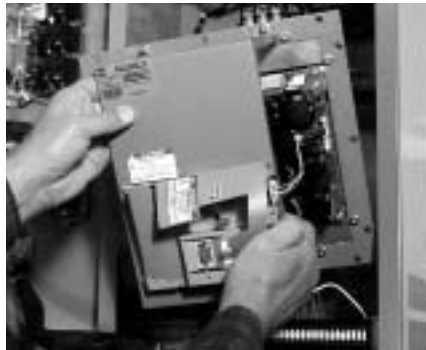
Figure 26: Remove Power Converter
