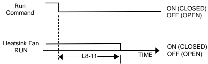
Fig. 84 Heatsink Cooling Fan Operation Timing Diagram
