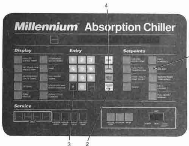
FIG. 9 - KEYPAD - PROGRAMMING "HOLIDAY" SETPOINT
