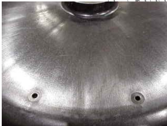
Figure 30 - Fan Drain (Prior Serial Number 5200F)
