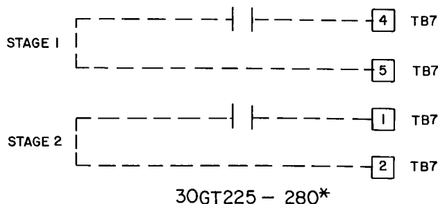
Fig. 22 - Demand Limit - Two External Switch Inputs
