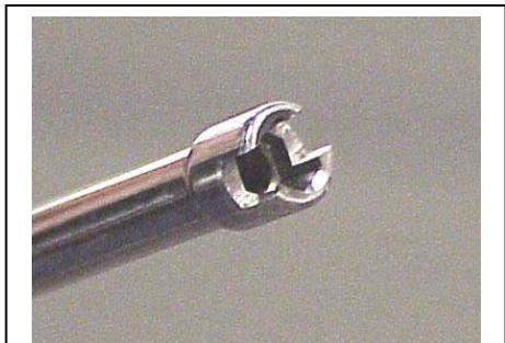
Figure 7. Slotted Nut Driver Core Removal Tool (Hand-made)
