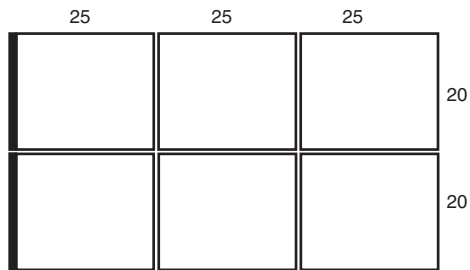
Unit Size 21 Flat Filter Section (6) 20 x 25
