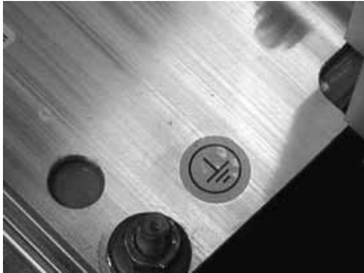
Figure 3-3: Grounding Terminal on Mounting Plate
