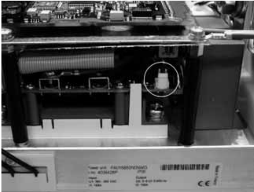
Figure 4-5: Connection of Control Board Cable from the Power Board CORRECT: Terminal J2 (Lower)
