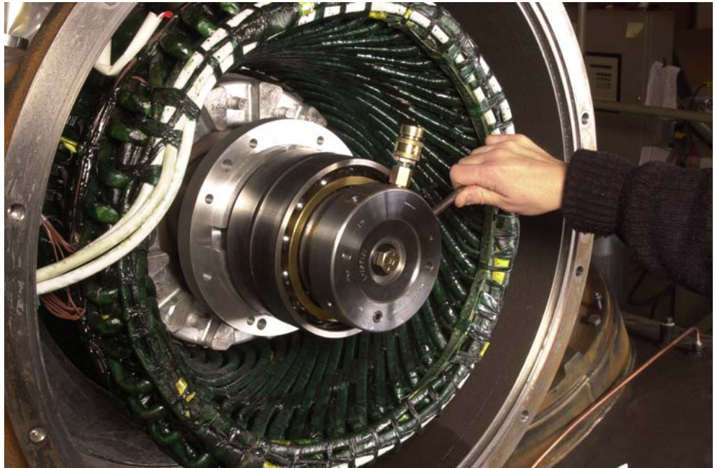
Figure 11: Tighten the hydraulic assembly nut using the rod provided with the nut
