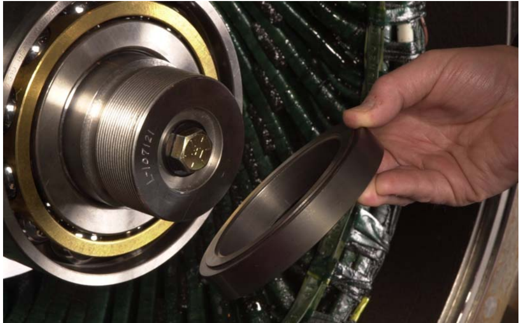
Figure 9: Install the hardened spacer ring as shown. The raised face of the ring goes against the bearing inner race
