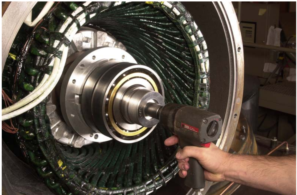
Figure 7: Use an impact wrench to tighten the cap screw on the shaft extension. Torque to 150-200 ft-lbs
