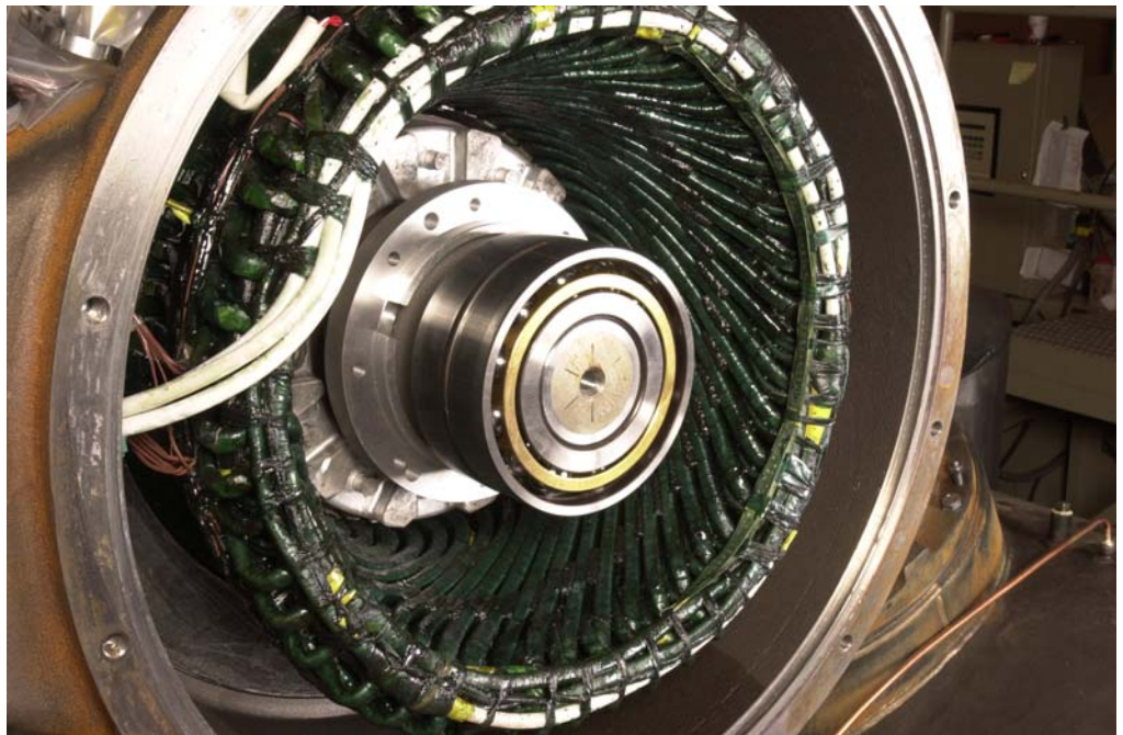
Figure 3: Remove the second bearing from the heater and install it onto the shaft. Note: The oil grooves on the outer race of each bearing must face one another, but do not have to align with each other.
