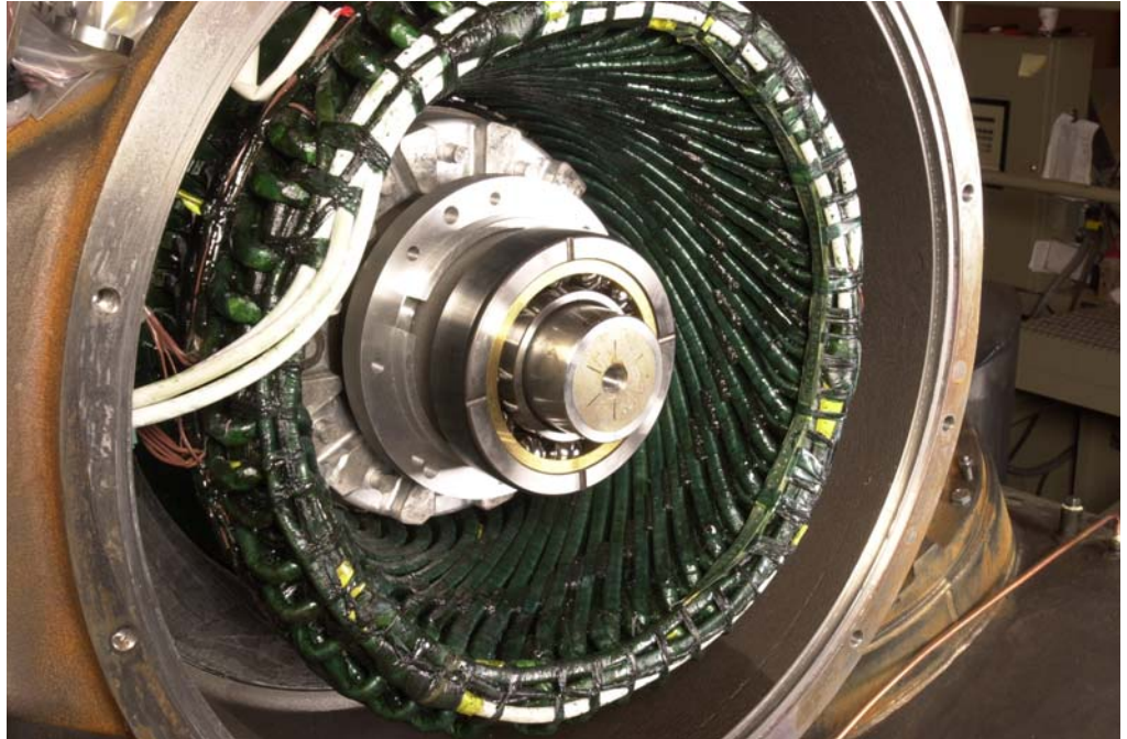
Figure 2: After heating the bearing, slide the first half onto the shaft as shown. Note the center feed grooves in the outer race which provide oil feed to the bearings.
