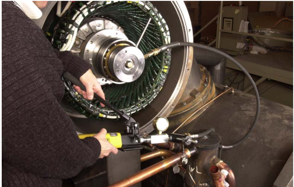
Figure 12: Bleed the assembly and then pressurize the assembly nut to 2700 to 2800 psi
