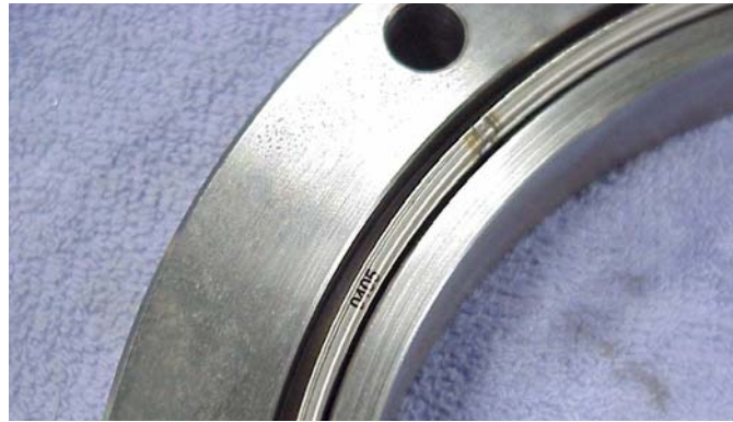
Figure 16: Photo of crush ring showing the laser-etched four-digit number
