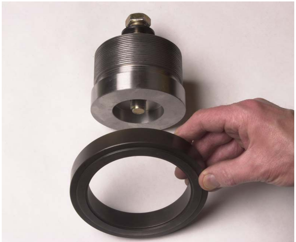
Figure 5: TOL01550 - REQUIRED for servicing the thrust bearings on CVHF1470 and CVHF1720 compressors. This tool contains the hardened spacer, threaded shaft extension, hardened washer, and cap screw
