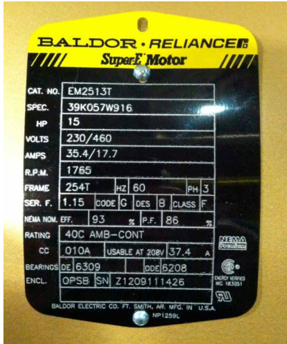
FIGURE 100 - TYPICAL MOTOR DATA/NAME PLATE
