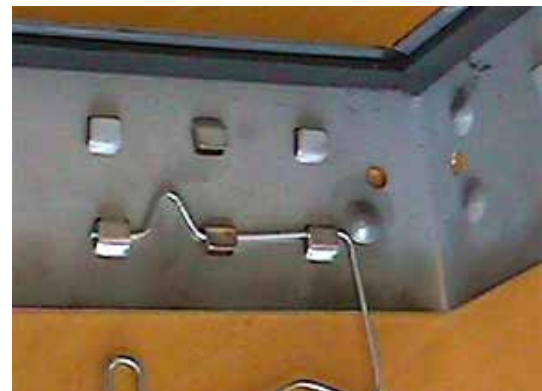
FIGURE 88 - CORRECTLY INSTALLED LATCH PIN (P/N 026-35788-604)
