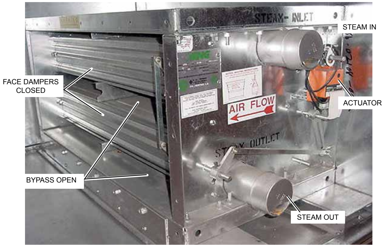
FIGURE 60 - IFB COIL (HORIZONTAL TUBES AVAILABLE WITH STEAM AND HOT WATER)
