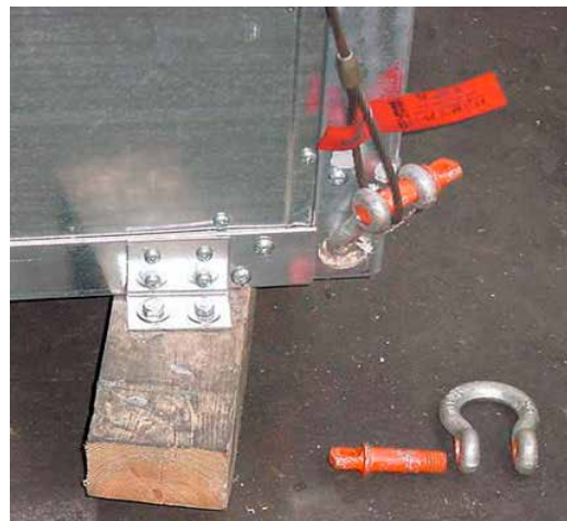
FIGURE 12 - PROPER LIFTING WITH SHACKLE WITH CORNER CONNECTOR CORNERS
