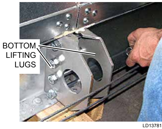
FIGURE 62 - FASTEN BOTTOM LIFTING LUGS
