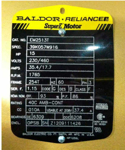
FIGURE 100 - TYPICAL MOTOR DATA/NAME PLATE
