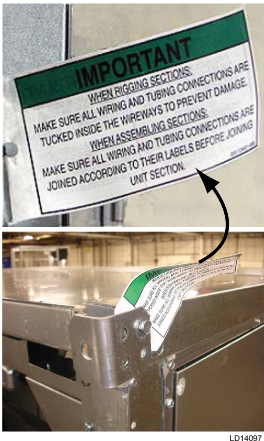
FIGURE 60 - REMOVE AND REPOSITION SHIPPING SPLIT ANGLE
