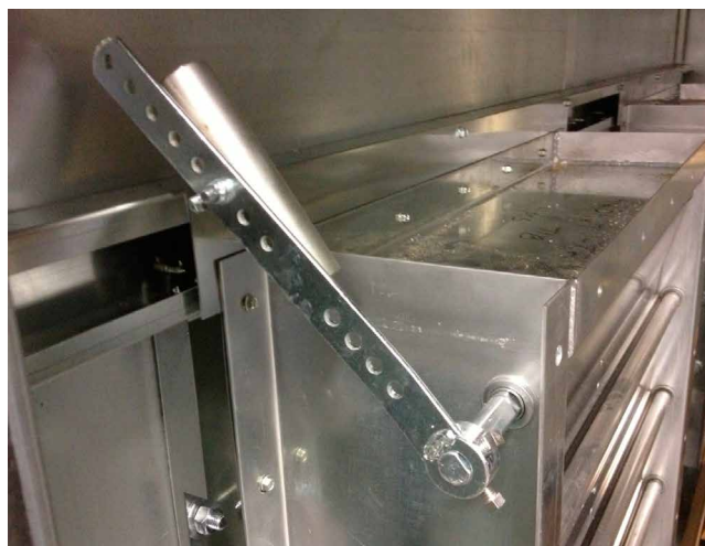
FIGURE 76 - COUNTERBALANCE UNLOCKED FOR START-UP
