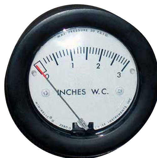
FIGURE 83 - MINIHELIC FILTER GAUGE
