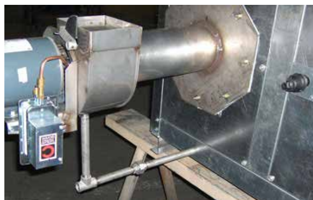
FIGURE 30 - SET ID FAN DAMPER
