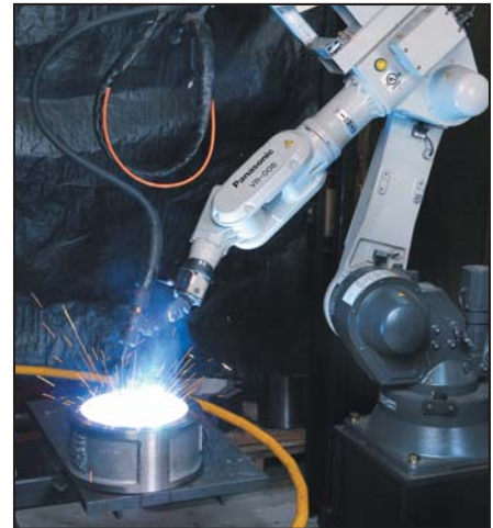
A robotic welding system applies a Stellite deposit onto a 10" Class 150 Wafer Type PW body seat with GMAW process.
