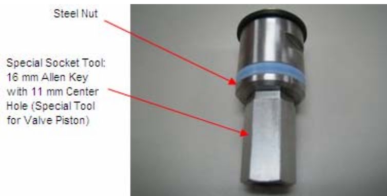
Figure 4: Danfoss 16 mm Allen Key Inserted into a Steel Nut
