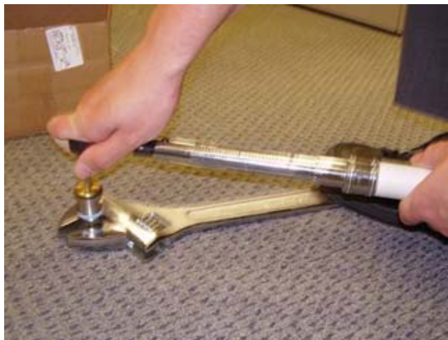
Figure 9: Torque to 25 N·m (18.5 lb-ft)
