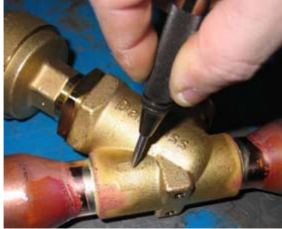
Figure 3: Reworked Valve with a Punch Mark
