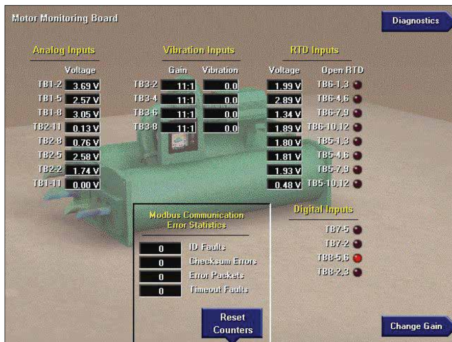
FIGURE 109 - MOTOR MONITORING BOARD DIAGNOSTIC SCREEN
