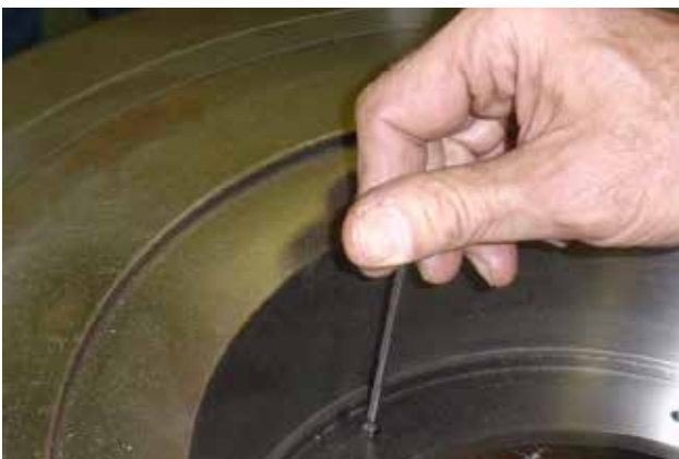
FIGURE 69 - TIGHTEN SET SCREWS LD13194
