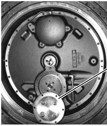
FIGURE 33 - LOW-SPEED THRUST BEARING REMOVED
