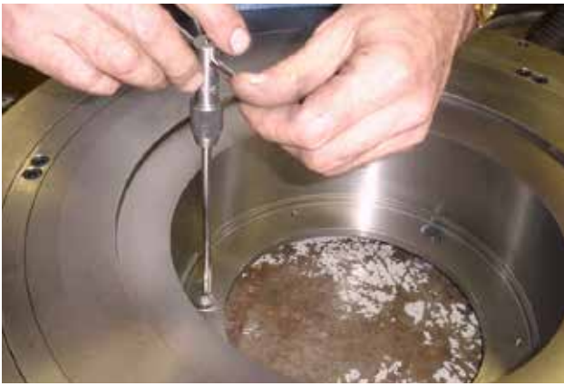
FIGURE 67 - TAP THE DRILLED HOLES LD13192
