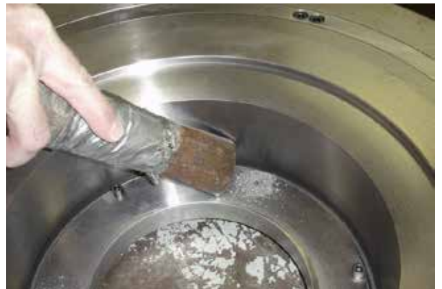
FIGURE 66 - REMOVE METAL DEBRIS
