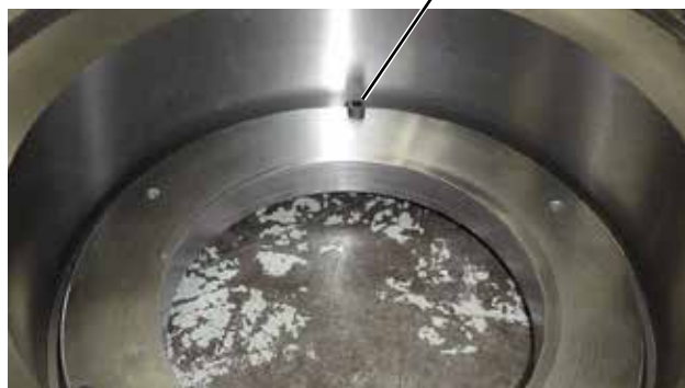
FIGURE 64 - DRILL GUIDE/FIXTURE INSTALLED
