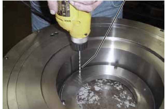
FIGURE 65 - DRILLING NEW HOLES
