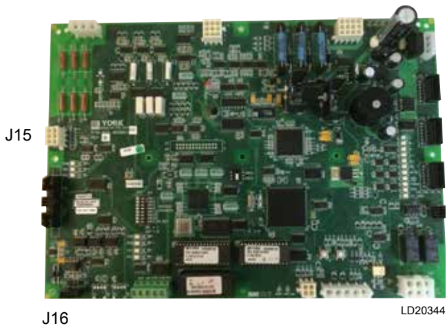
FIGURE 2 - VSD MODEL DRIVE LOGIC BOARD 031-02506-002, 031-02506-003
