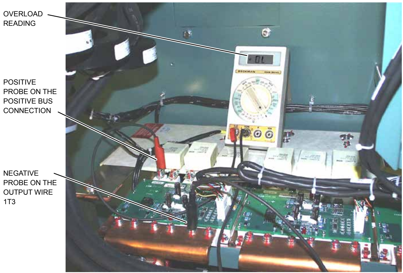
FIGURE 50 - 385/419/503/608/658/704/900 HP DRIVE IGBT MODULE VERIFICATION #1
