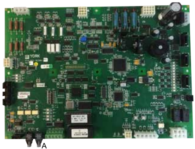
FIGURE 3 - VSD MODEL DRIVE LOGIC BOARD 031-02506-002, 031-02506-003 REVISION 'F' OR LATER
