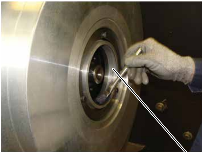
FIGURE 74 - BALANCE PISTON SEAL LUBRICATION
