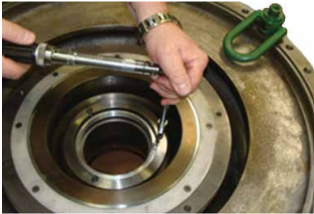
FIGURE 60 - EYE SEAL REMOVAL
