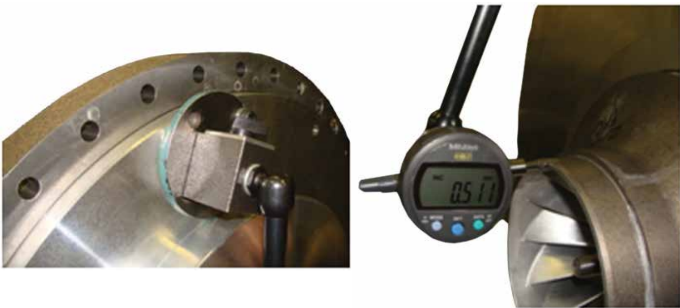
FIGURE 99 - ROTOR AXIAL CLEARANCE CHECK
