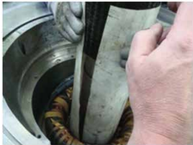
FIGURE 90 - MOTOR / STATOR PROTECTION
