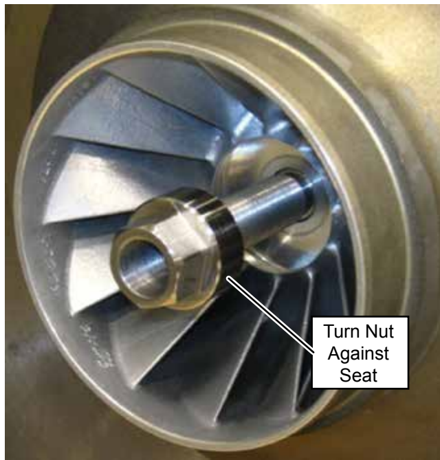
FIGURE 75 - IMPELLER MOUNTING NUT
