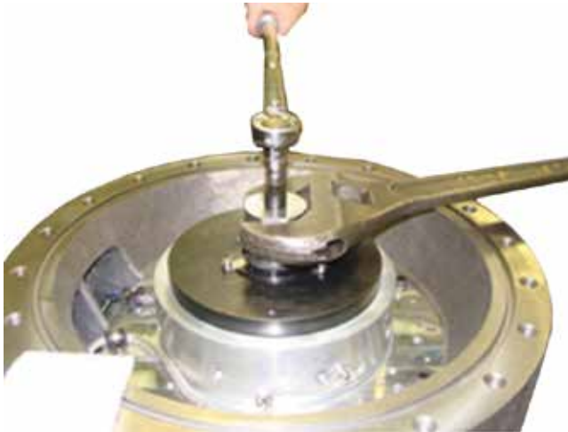
FIGURE 94 - THRUST RING RETAINER BOLT
