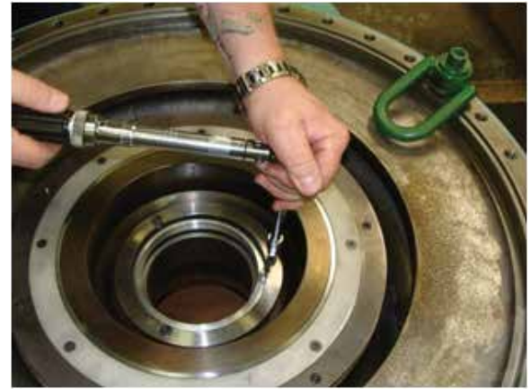
FIGURE 66 - EYE SEAL TORQUE
