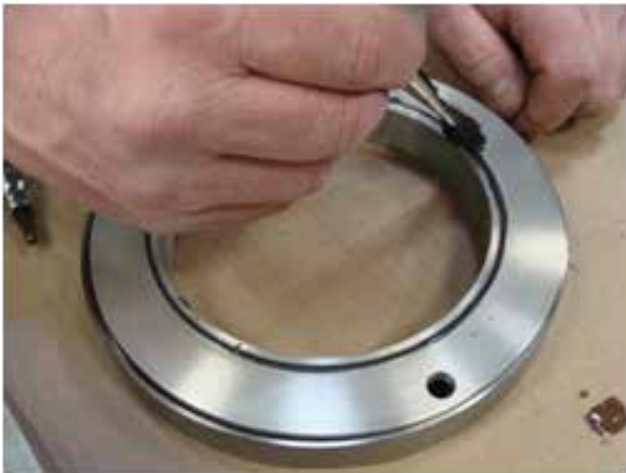
FIGURE 79 - SEAL RING LUBRICATION
