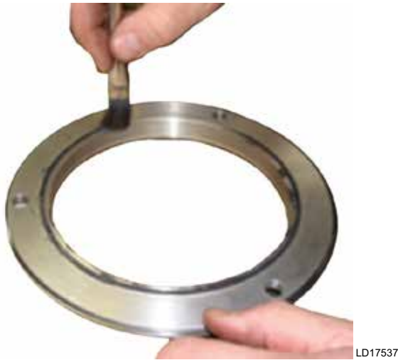
FIGURE 64 - EYE SEAL LUBRICATION
