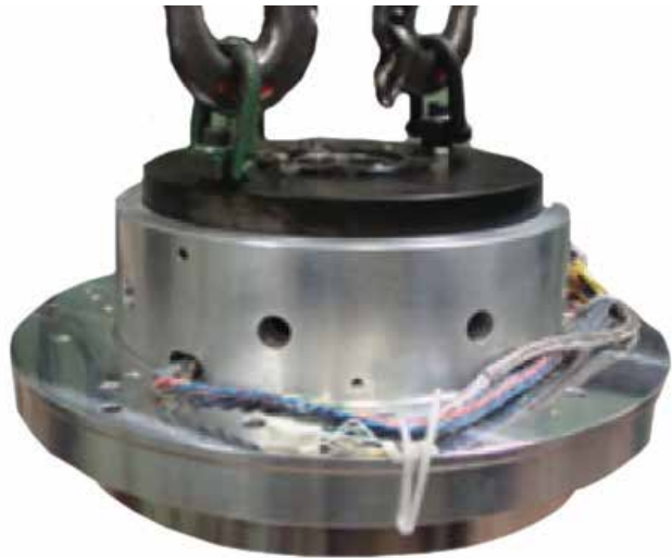
FIGURE 97 - Z2 BEARING RIGGING
