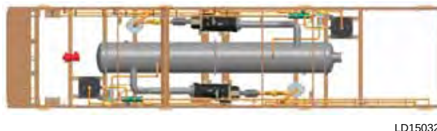
FIGURE 9 - 2-PASS EVAPORATOR STANDARD ARRANGEMENT
