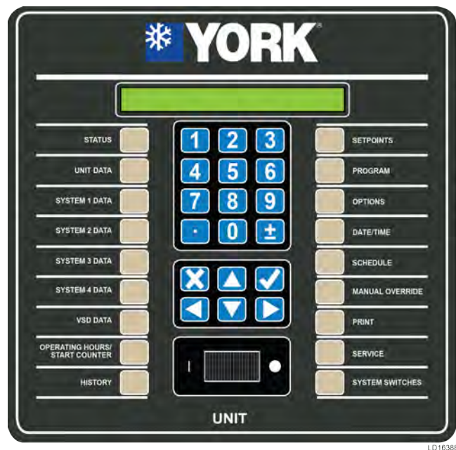
FIGURE 5 - CONTROL CENTER USER INTERFACE
