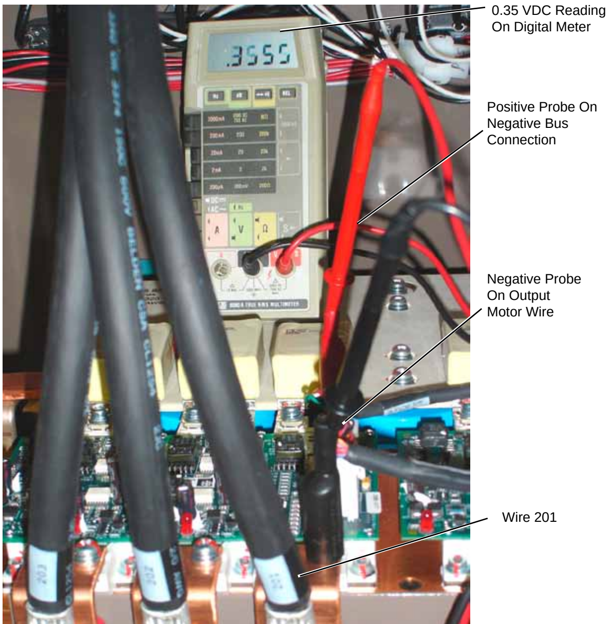
FIGURE 86 - IGBT MODULE VERIFICATION #1
