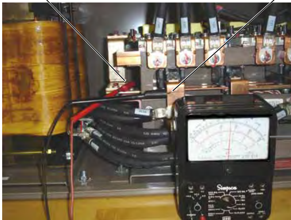
FIGURE 92 - SCR / DIODE MODULE VERIFICATION #3
