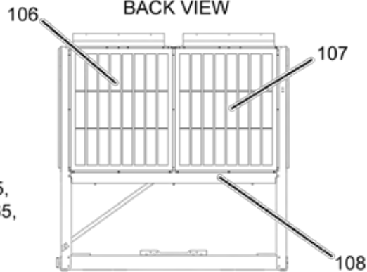
FIGURE 69 - TOP SECTION: LOUVERED ENCLOSURE KIT COMPONENTS - MODELS 0178/0588, 0195/0665, 0198/0688, 0213/0743 - 0245/0865, 0263/0963, 0275/0965
